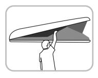
5 Unlock the gas springs, and close the tent completely.
