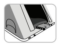
3 Pull the tent down using the closing strap. Don't close the tent completely, leave it about 20cm opened, and use the rotary knob to lock the gas springs.
