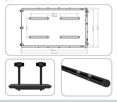
4 Open up the side doors and insert the two hand grip screws through the holes on the bottom, so that the roof bar lies between them. Do this for all the four ends of the two roof bars.
